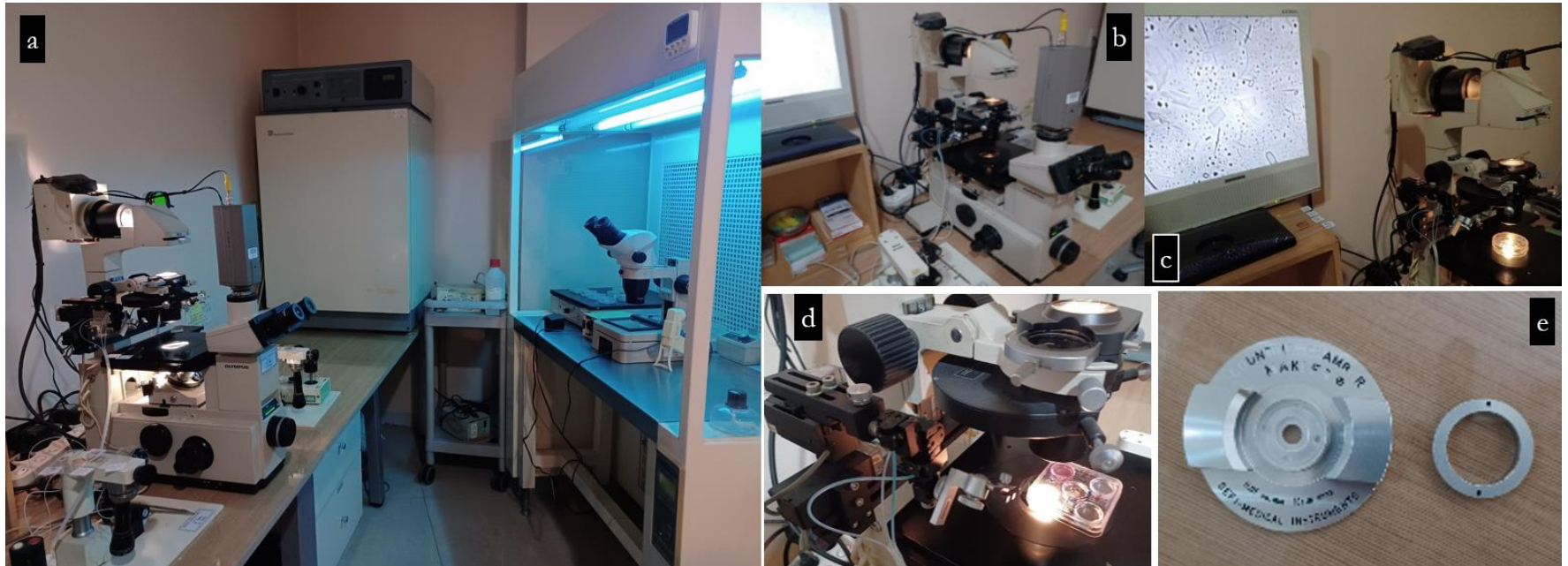
Figure 1. Lab equipment: (a) at right, a stereomicroscope, a laminar air flow clean bench with UV and heat template; (b) a stereomicroscope connected to an LCD monitor for viewing; (c) Moderna culture dish on the stereomicroscopic plate with video monitoring; (d) 5 well culture dishes on the plate; (e) a Makler Counting Chamber.
